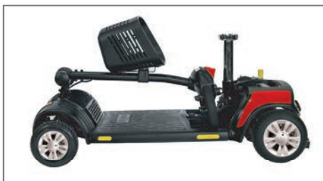
Detachable battery pack and adjustable angle tiller.
